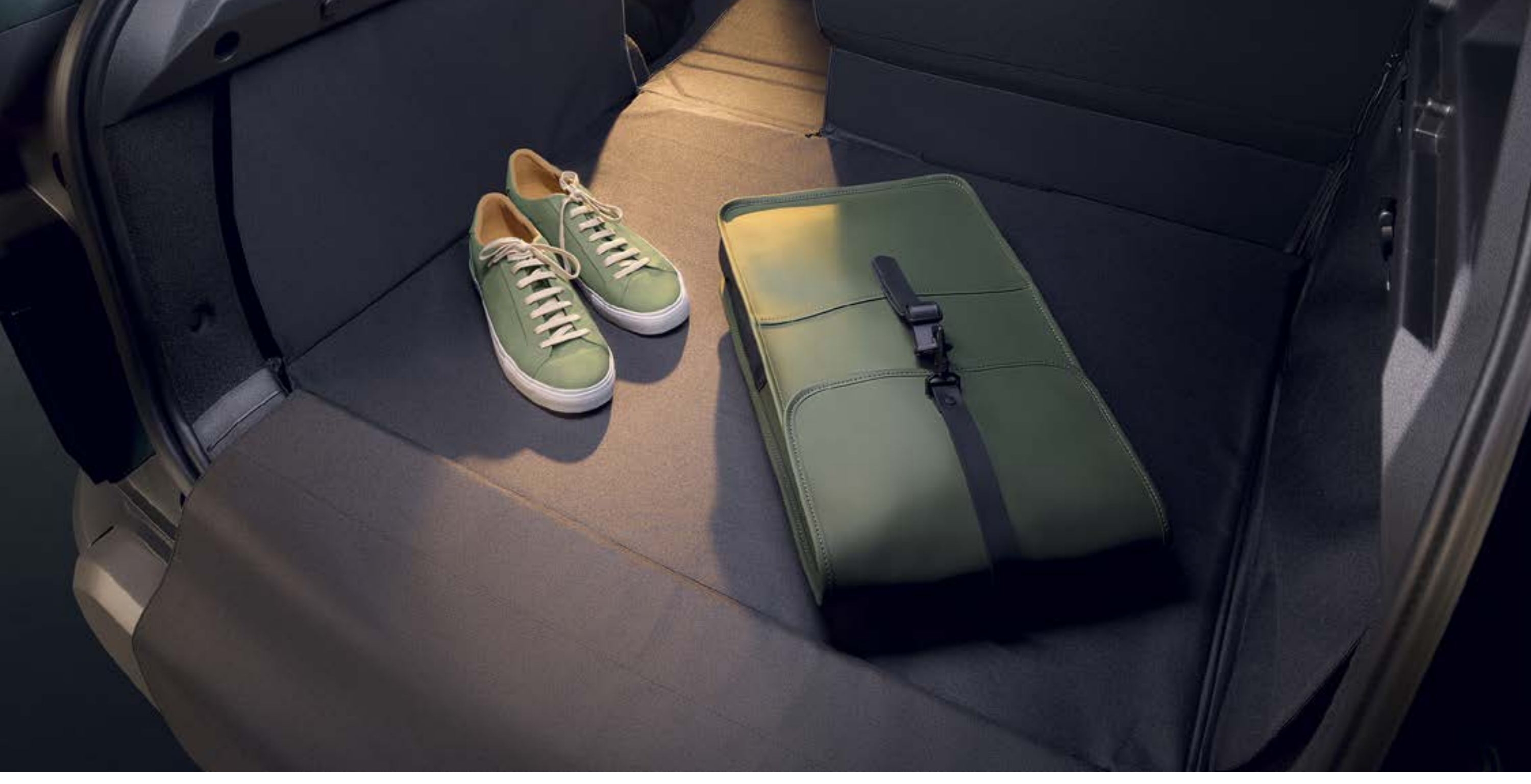
EasyFlex modular luggage compartment protection Non-slip and waterproof protection provides a practical solution for carrying loads in all weather conditions. Thanks to the adaptable structure, it covers all the luggage compartment surface when rear seats are folded.
